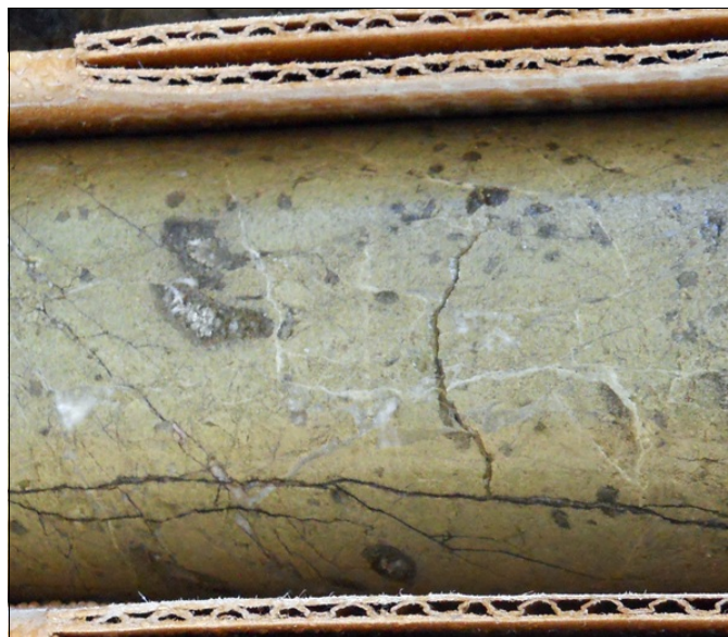
Greenish colored propylitic alteration with calcite veining in andesitic volcanics at the Rosemont deposit, Pima County, Arizona (Photo taken Jan Rasmussen, September 2012).
