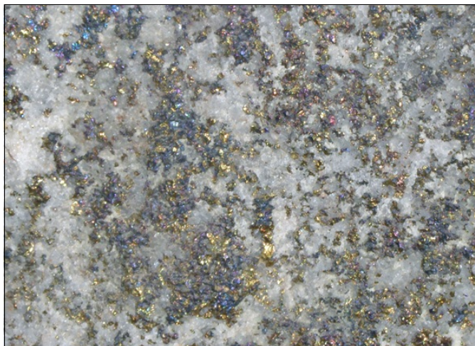
Chalcopryite-bornite-quartz vein from the Dos Pobres Copper Deposit near Safford, Arizona (Photo taken by David Briggs).
